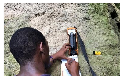
Doctorant at the Cheikh Anta Diop University, Senegal, measuring K, Th, U concentrations
